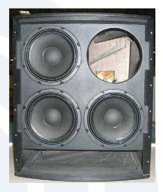
The picture above shows what the S410s looks like with the grill and top right woofer removed. Place the new woofer (part #0011737) where the old one was. Follow the same steps as above, but backwards 4 to 1. Power up the S410s and the new woofer should now be pumping out glorious lows. Awesome, you just replaced a 10" woofer!
